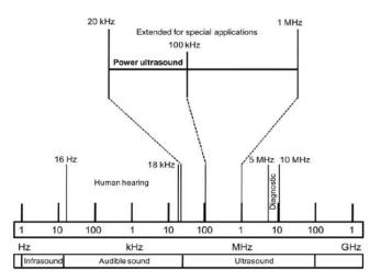
**Fig. 1**: Frequency ranges of sound indicating infrasound (1 Hz-16 Hz), human hearing (16 Hz-18 kHz), power ultrasound (20 kHz-100 kHz), extended for special applications (20 kHz-1 MHz) and diagnostic ultrasound (5 MHz-10 MHz)<sup>6</sup>.
