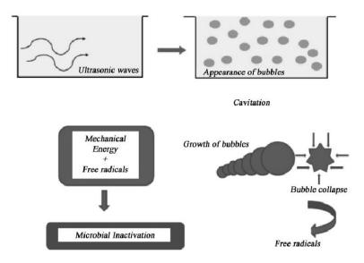
Fig. 2. Ultrasonic waves and the cavitation phenomenon<sup>13</sup>
