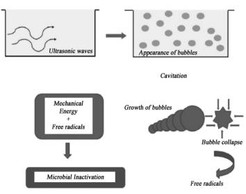
Fig. 2: Ultrasonic waves and the cavitation phenomenon<sup>13</sup>
